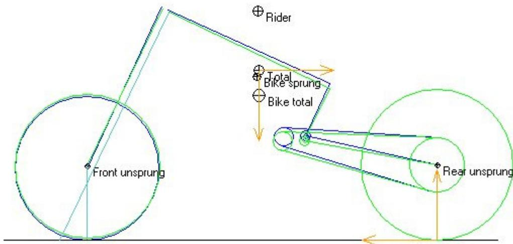
There are no forces on the front wheel. The forces on the CoG and the rear wheel are in balance, as can be seen at the orange arrows.
